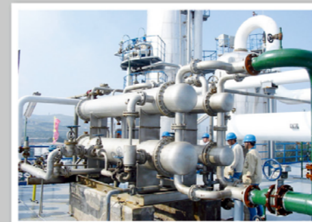
丁辛醇装置精馏真空系统 Rectification Vacuum System for Oxo Alcohol Device
