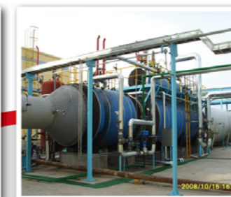
己二酸废气废液焚烧单元 (新疆天利) Incineration unit of adipic acid waste gas (Xinjiang Tianli)
