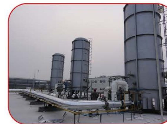
火炬气回收与排放地面火炬一体化装置 (大连恒力) Integrated ground flare unit for recovery and discharge of flare gas (Dalian Hengli)
