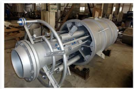
伴烧内燃蓄热火炬头 Flare tip with internal combustion heat storage
