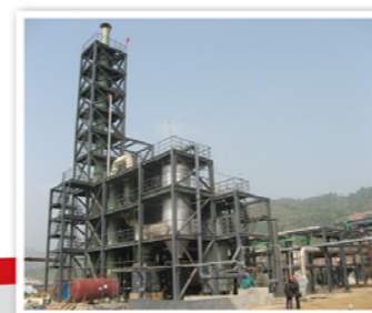
蛋氨酸废气废液焚烧单元 (重庆紫光) Incineration unit of methionine waste liquid and waste gas (Chongqing Ziguang)
