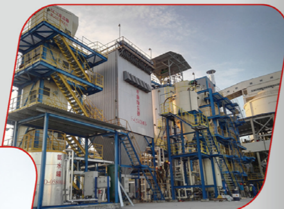
煤化工危险废物焚烧系统 (神华宁煤) Coal chemical hazardous waste incineration system (Shenhua Ningxia Coal)
