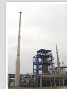
树脂废气废液焚烧单元 (金陵帝斯曼) Incineration unit of resin waste gas and liquid (Jinlin DSM)
