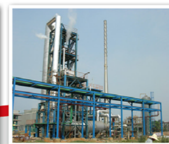
WSA 酸性气焚烧单元 (宝钢) WSA unit of H 2 S gas (Baosteel)
