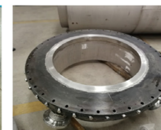
激冷环维修前后 Quench ring before and after maintenance
